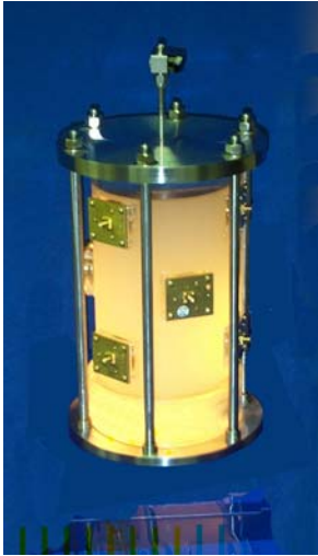
Figure 4: A module of the new 4.5 litre detectors with an active mass of 60g. The container is entirely fabricated from acrylic. Each module is equipped with 9 piezo-electric sensors for event localization.
