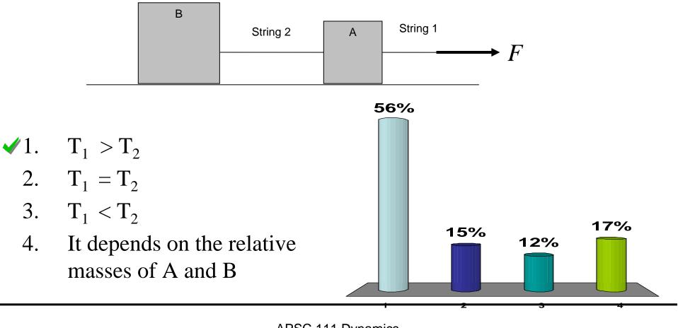
This can be answered intuitively, or by using free body diagrams. Since the system is frictionless, with a constant force there will be a constant acceleration, which is the same for each block as they are attached. String 1 has a tension due to the combined mass of A and B, String 2 has only the mass of B, so the tension  $T_2$  is always less than  $T_1$
